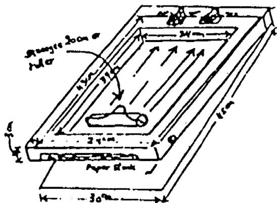
The frame is firmly hinged to a wooden base which supports the duplicating paper to prevent the screen and stencil from shifting while printing is being done. If the whole process is done carefully, the results will be as readable as that of copies duplicated on a manual duplicating machine.
