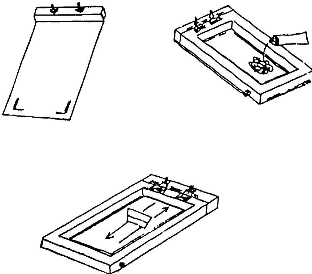
After printing, each separate sheet is removed to dry for at least thirty minutes, or it is separated from the next sheet by old paper to prevent ink from soiling the back of the next page.
